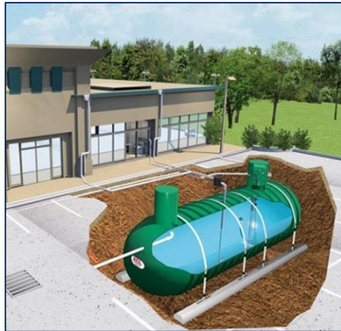
Figure 3.4 - Example of Rainwater Harvesting System
